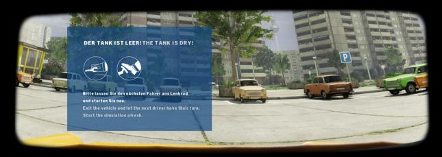
Distorted image, which gets projected on the windshield of the car so the driver gets an undistorted view.
